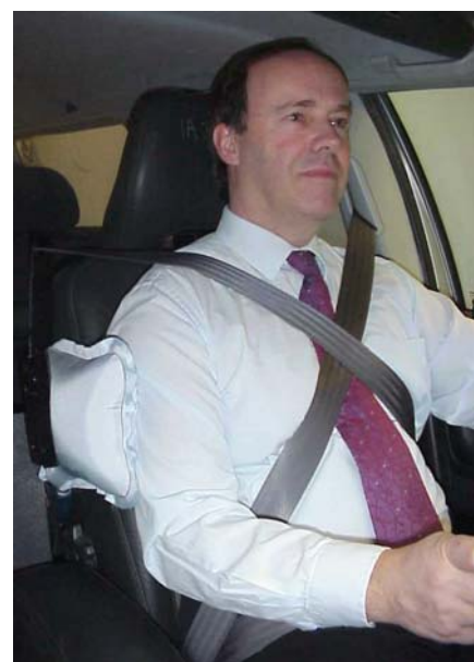
Figure 1. The 3+2 point belt system and an inboard torso side support (inflated bag) implemented in a car.
